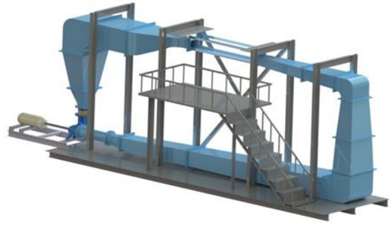
Figure 2. General schematic of the closed circuit free surface water tunnel of the Babol Noshirvani University of Technology
