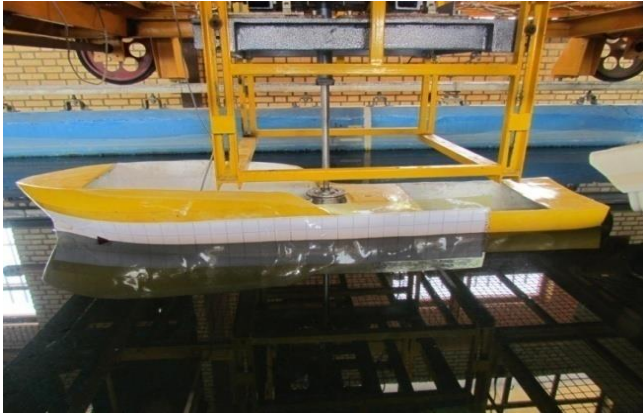
Figure 3. Ship model attached to dynamometer
