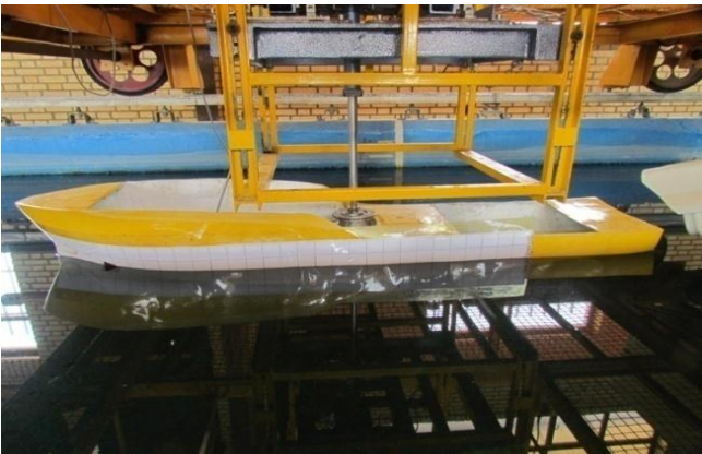
Figure 3. Ship model attached to dynamometer
