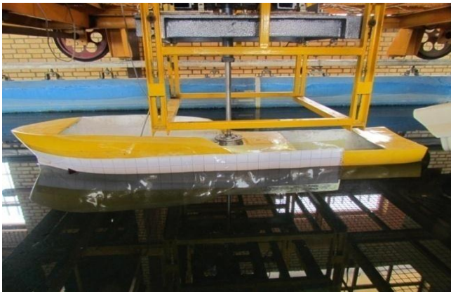
Figure 3. Ship model attached to dynamometer
