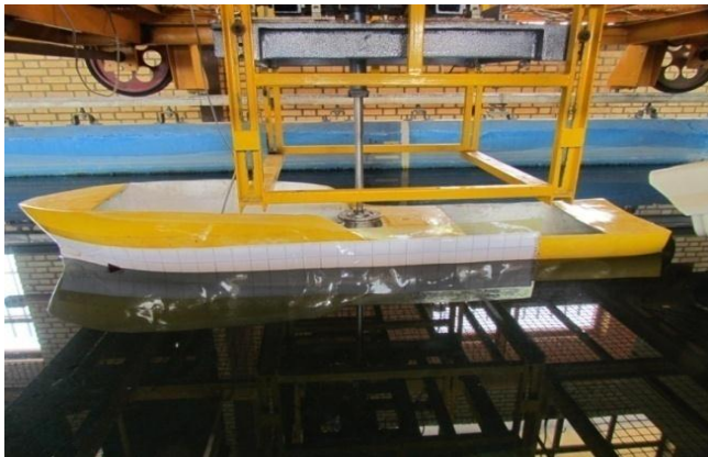
Figure 3. Ship model attached to dynamometer
