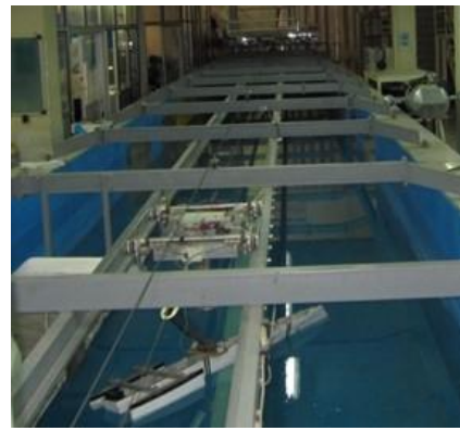
Figure. 3 Towing tank facilities of the Marine Research Centre (MRC) at the Sharif University of Technology (SUT)
