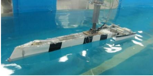
Figure. 6 Model during resistance test under head sea condition (model speed=0.5 m/s)
