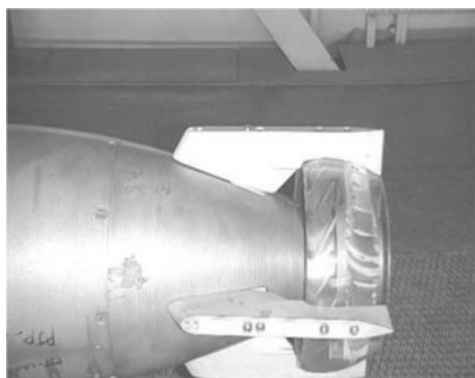
Figure.1 Pump jet propulsion of underwater marine vehicle[1]
