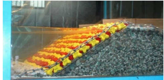
Figure 1 Geometry of breakwater built in the lab [16]
