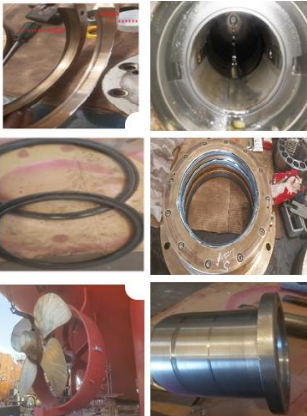
Figure 12. Stern tube aft ring seal box [13].
