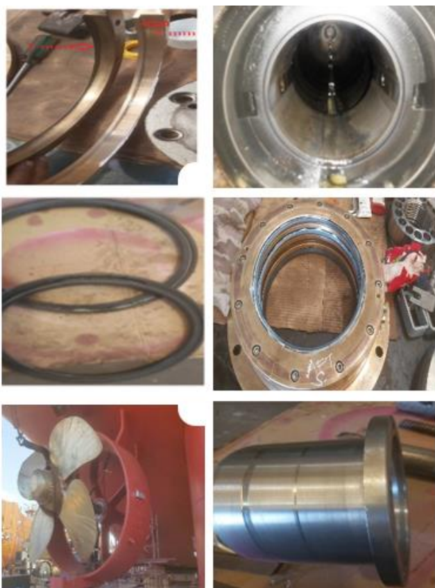
Figure 12. Stern tube aft ring seal box [13].
