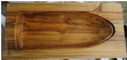
Fig. 5. Initial mold used for hull model construction
