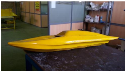
Fig. 6. Photograph of the completed hull model
