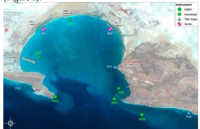
Figure 1. Positioning of measurement devices at the end of the sixth month (Ports and Maritime Organization Monitoring and Modeling Project)
