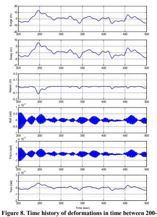
Figure 8. Time history of deformations in time between 200-500 sec,  $\Delta t = 0.68$ sec
