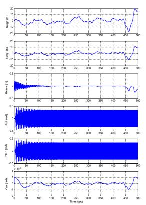
Figure 15. Time history of deformations,  $\Delta t = 0.7 \text{sec}$
