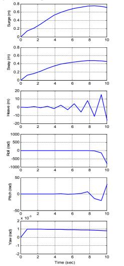
Figure 19. Time history of deformations sec,  $\Delta t = 0.78 \text{ sec}$
