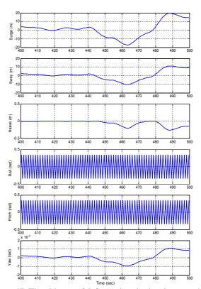
Figure 17. Time history of deformations in time between 400-500 sec,  $\Delta t = 0.7 \, \text{sec}$
