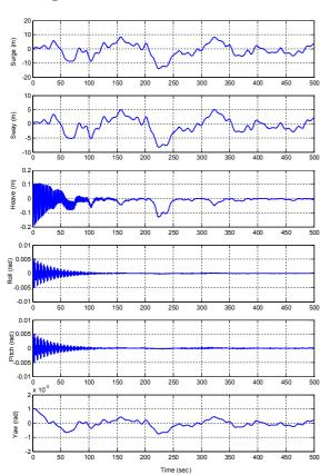
Figure 3. Time history of deformations,  $\Delta t = 0.67 \text{sec}$
