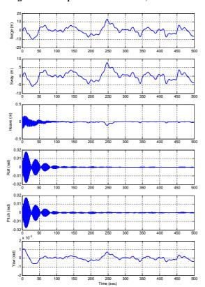
Figure 7. Time history of deformations,  $\Delta t = 0.68 \text{sec}$
