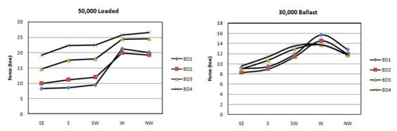
Figure 4. Variation of Forces on fenders due to variation of wave direction
