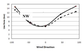
Figure 3. Variation of tension in mooring line against the wind direction for two wave directions. Solid lines are for fully loaded condition and dashed lines are for ballast condition
