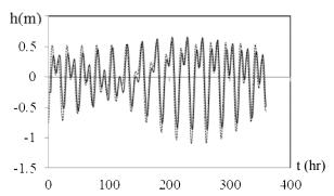
Figure 6. Comparison between simulated (dashed line) and measured (solid line) water levels at Lavan Island (1<sup>st</sup> to 15<sup>th</sup> of January 2009)
