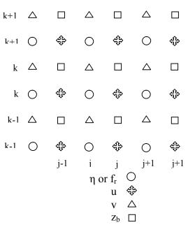
Figure 2. Finite difference grid arrangements in ADI scheme
