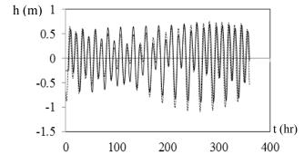
Figure 5. Comparison between simulated (dashed line) and measured (solid line) water levels at Kangan (1<sup>st</sup> to 15<sup>th</sup> of January 2009)
