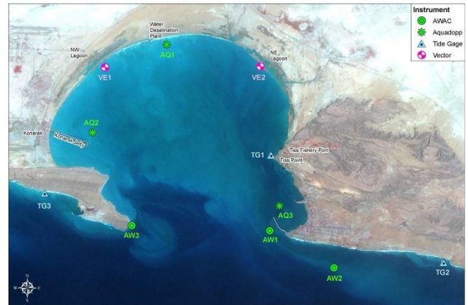
Figure 3. Locations of deployed instruments in February 2007 (AW refers to an AWAC, AQ refers to an Aquadopp and TG refers to a Tide Gauge)
