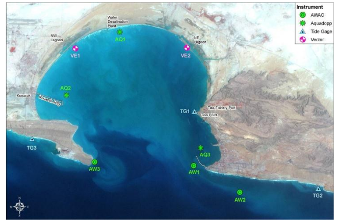
Figure 3. Locations of deployed instruments in February 2007 (AW refers to an AWAC, AQ refers to an Aquadopp and TG refers to a Tide Gauge)
