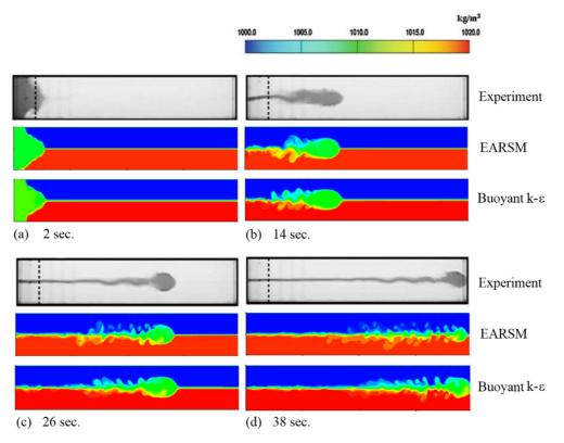
Figure 4. Temporal evolutions of an intrusive gravity current for case 1, where experimental results of Sutherland et al. [35] are compared with simulated density contours based on buoyant k-ε and EARSM turbulence closures.
