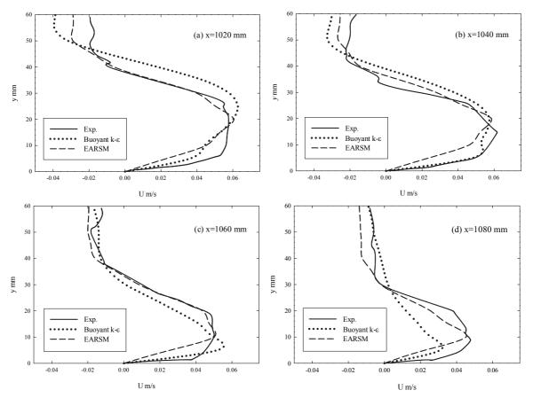
Figure 10. Velocity profiles of turbulence models and measured values at (a) x=1020mm, (b) x=1040mm, (c) x=1060mm and (d) x=1080mm in experiments of Zhu et al. [36]
