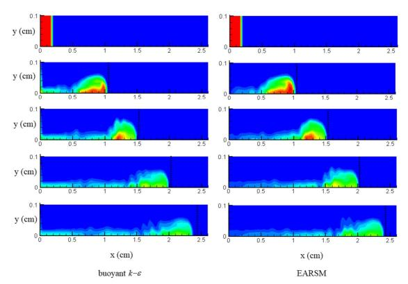
Figure 8. Results of simulated salinity distribution for EARSM and buoyant k-ε turbulence closures at 0, 23, 36, 52 and 62s in experiments of Zhu et al. [36]. The dotted line in the frames is the experimentally reported location of the nose of the gravity
