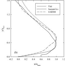
Figure 2. Velocity profiles of turbulence models and measured values at (a) x=0.9m and (b) x=2.4m in experiment of Gerber [34]
