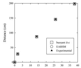
Figure 5. Traveling distance of intrusive gravity current as a function of time in case 1, for simulated values of buoyant k- ε and EARSM closures and measured values [35]
