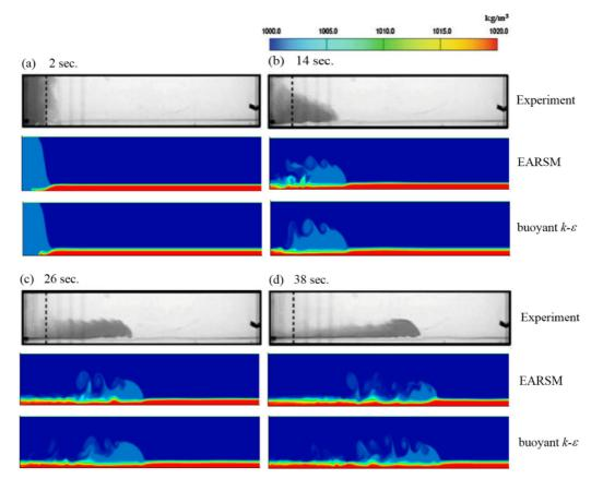
Figure 6. Temporal evolutions of an intrusive gravity current for case 2, where experimental results of Sutherland et al. [35] are compared with simulated density contours based on buoyant k-ε and EARSM turbulence closures.
