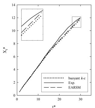
Figure 9. Comparison of front head position for EARSM and buoyant k-\varepsilon turbulence closures with measured values of Zhu et al. [36]
