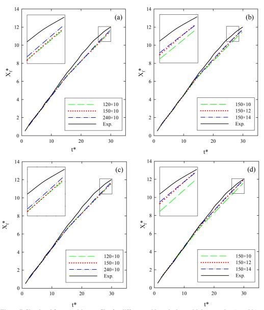
Figure 7. Simulated front position profiles for different grid resolutions with buoyant k-ε (a and b) and EARSM (c and d) turbulence closures in experiment of Zhu et al. [36]
