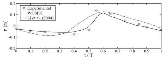
Figure 5. Comparison of computed water surface elevations by SPH with experimental and numerical data of Li et al. [5] for WG3 (x=3.81 m)
