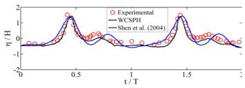
Figure 9. Comparison of estimated water surface elevations by WCSPH, experimental data of Ohyama et al. [22] and numerical data of Shen et al. [6] for case 2
