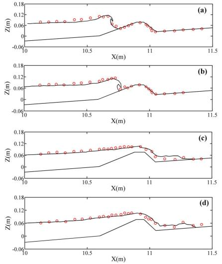
Figure 15. Comparisons of free surface evolution between measurement data (Red circles)[1] and WCSPH model (black solid lines) for case 2. Simulated free surface at a) t = 2.95 s, b) t = 3.01 s, c) t = 3.22 s, and d) t = 3.34 s.
