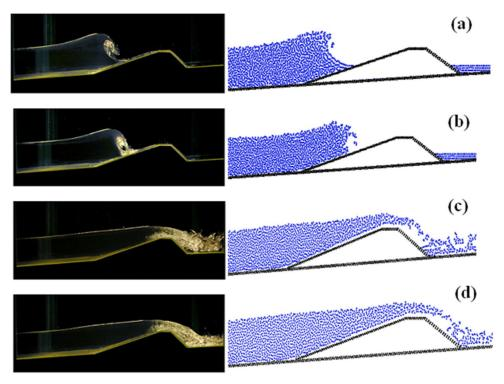
Figure 14. Comparisons of free surface evolution between laboratory images (left)[1] and WCSPH particles snapshots (right) for case 2 at a) t = 2.95 s, b) t=3.01 s, c) t= 3.22 s, and d) t= 3.34s.
