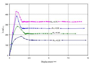
Figure 11. Failure mechanism No. 1. Typical numerical pullout response of suction caissons in weak clay under drained conditions (Kaolinite clay, drained condition, L=600 mm, D=100 mm, c=0.1 kPa,  $\varphi=27.8^{\circ}$ ,  $\psi=0$ , E=1 MPa, v=0.35).
