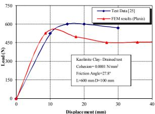
Figure 4. Verification of numerical results against experimental data for suction caisson models in clay under drained conditions (Kaolinite clay, drained condition, L=600 mm, D=100 mm, c =1 kPa,  $\varphi$  =27.8°,  $\psi$ =0, E=1 MPa, v=0.35).
