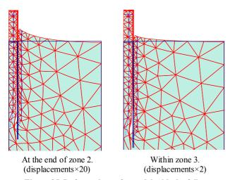
Figure 25. Deformations of a model with the failure mechanism No. 4 at different stages of pull-out (sand, undrained condition, L=600 mm, D=100 mm, c =0 kPa,  $\varphi$  =41°,  $\psi$ = 11°, E=25 MPa,  $\nu$ =0.3).
