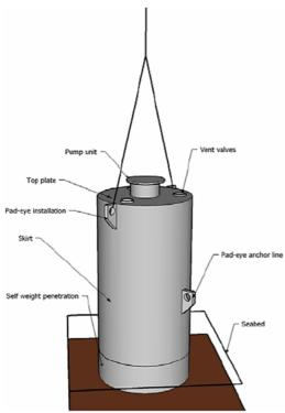
Figure 1: Schematic view of a suction caisson [3]
