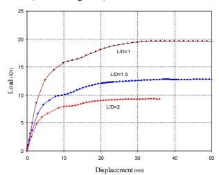
Figure 16. Failure mechanism No. 2. Typical numerical pullout response of suction caissons in clay under drained conditions (Kaolinite clay, drained condition, L=600 mm, D=variable, c=1.5 kPa,  $\varphi=27.8^{\circ}$ ,  $\psi=0$ , E=1.5MPa, v=0.35).
