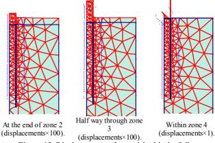
Figure 13. Displacements of a model with the failure mechanism No. 1 (model in Figure 11 with  $R_{ini}$ =0.5) at different stages of pull-out.
