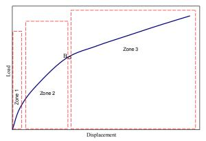
Figure 23. Schematic load-displacement response with the failure mechanism No. 4.
