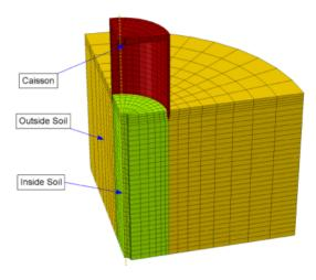
Figure 5. A view of the 3D Abaqus finite element model of a suction caisson.
