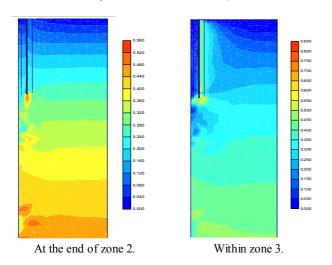
Figure 26. Relative shear stresses at different stages of pull-out in a model with the failure mechanism No. 4 (sand, undrained condition, L=600 mm, D=100 mm, c =0 kPa,  $\varphi$  =41°,  $\psi$ = 11°, E=25 MPa, v=0.3).
