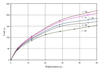
Figure 24. Failure mechanism No. 4. Typical numerical pullout response of suction caissons in sand under undrained conditions (Oklahoma sand, undrained condition, L=194 mm, D=110 mm, c=0 kPa,  $\varphi=$ variable,  $\psi=\varphi$  -30° for  $\varphi>$ 30°,  $\psi=$ 0° for  $\varphi\leq$ 30°, E=25 MPa, v=0.3).
