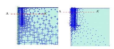
Figure 7. Variation of pore water pressure with an undrained model prior to the pull-out (in left where hydrostatic pressures are given and the water surface is also shown) and after the pull-out loading (in right where the excess pore pressures are shown and they gradually dissipate far away from the caisson.
