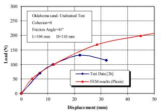
Figure 3. Verification of numerical results against experimental data for suction caisson models in sand under undrained conditions.
