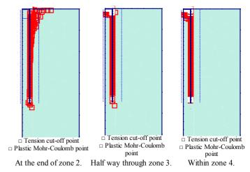
Figure 14. Plastic and tension cut-off points at different stages of pull-out in a model with the failure mechanism No. 1 (model in Figure 11 with  $R_{im}$ =0.5).
