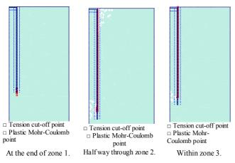
Figure 18. Plastic and tension cut-off points at different stages of pull-out in a model with the failure mechanism No. 2 (model in Figure 16 with L/D=6).
