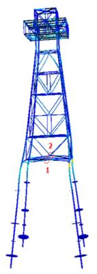
Figure 4. 3D view of the deformed shape of platform
