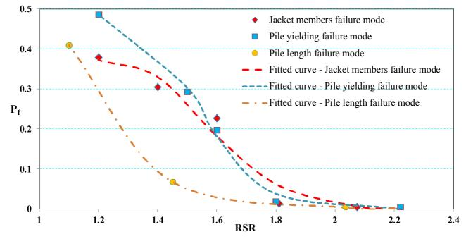
Figure 6. Presentation of the annual probability of failures for different values of RSRs
