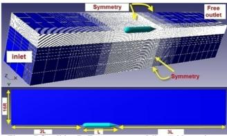
Figure 7.Condition B: Free stream modeling (without pipe wall effects)
