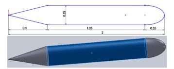
Figure 3. General configuration of the models
