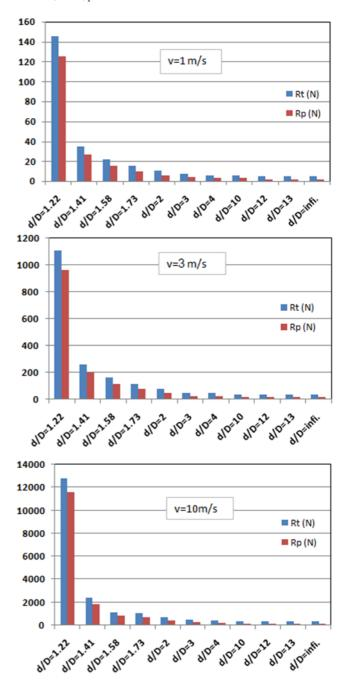
Figure 10. Total resistance and pressure resistance of AUV in several different d/D and speed
