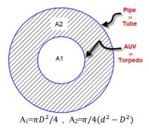
Figure 4. Cross section area of AUV and pipe (hatched area: water between AUV and pipe)
