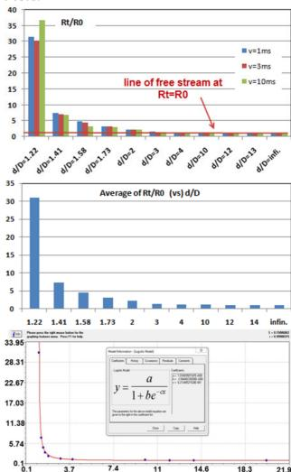
Figure 12. Ratio of total resistance to free stream resistance
