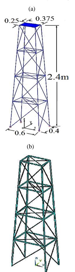
Figure 1. (a) The physical model and (b) finite element model of the jacket
