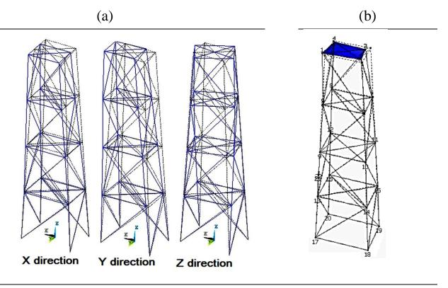
Figure 4. The first mode shape using (a) numerical modal analysis, (b) experimental modal analysis.
