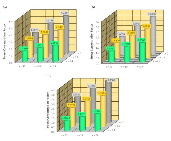
Figure 8. Effect of the  $\gamma$  on the SCFs under the 1<sup>st</sup> IPB loading condition ( $\theta = 45^{\circ}$ ,  $\beta = 0.4$ ): (a) Crown position, (b) Toe position, (c) Heel position
