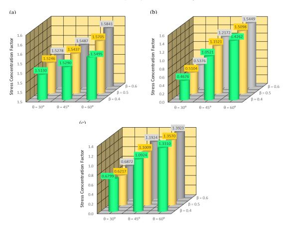
Figure 9. Effect of the  $\theta$  on the SCFs under the 1<sup>st</sup> IPB loading condition ( $\tau$  = 0.4,  $\gamma$  = 12): (a) Crown position, (b) Toe position, (c) Heel position
