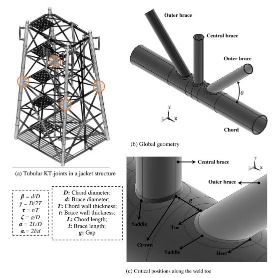
Figure 1. Geometrical notation for a simple uniplanar KT-joint
