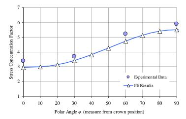
Figure 5. Distribution of chord-side SCFs along the central brace/chord intersection of uniplanar KT-joint:
