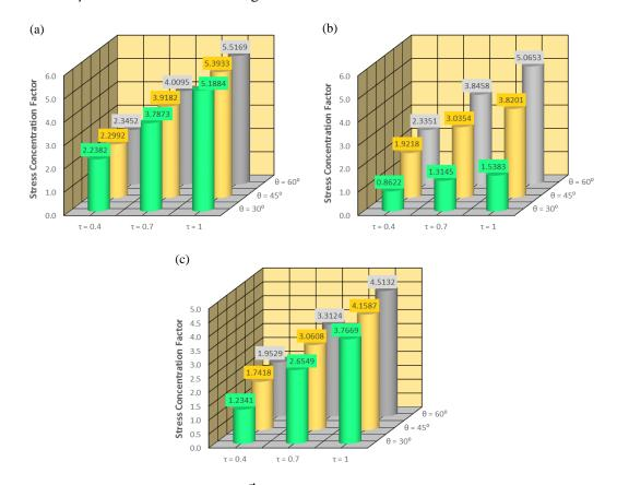
Figure 6. Effect of the  $\tau$  on the SCFs under the 1<sup>st</sup> IPB loading condition ( $\beta = 0.6, \gamma = 24$ ): (a) Crown position, (b) Toe position, (c) Heel position
