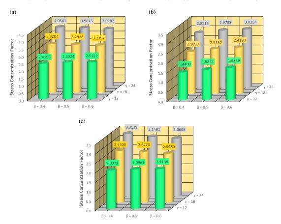
Figure 7. Effect of the  $\beta$  on the SCFs under the 1<sup>st</sup> IPB loading condition ( $\theta = 45^{\circ}$ ,  $\tau = 0.7$ ): (a) Crown position, (b) Toe position, (c) Heel position
