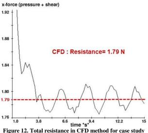
Figure 12. Total resistance in CFD method for case study validation
