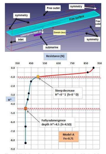
Figure 3. Variations of total resistance versus depth in (modeling in Flow Vision)[19]
