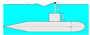
Figure 1. Snorkel depth in naval submarines
