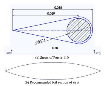
Figure 6: Cross section of struts
