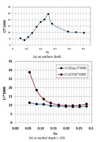
Figure 14. Resistance coefficients at surface draft and snorkel depth
