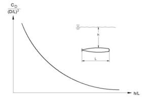
Figure 2: General variations of total Resistance coefficient versus submergence depth
