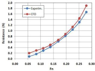
Figure 13. Comparison of the results of submarine bare hull resistance by CFD and experimental methods
