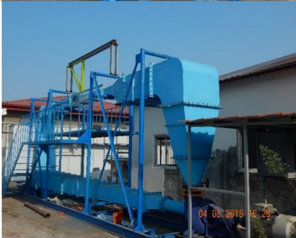
Figure 18. water tunnel built in Babol Noshirvani university of Technology
