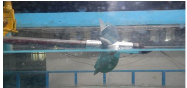
Figure 22. Dynamometer made that has been installed at test section
