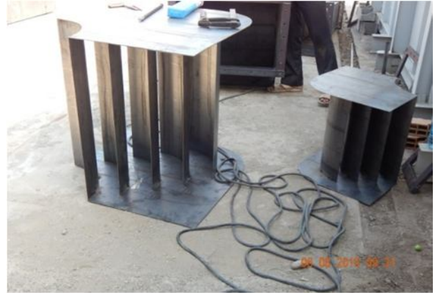
Figure 17. Initial view of the elbow and guide blades of the present water tunnel
