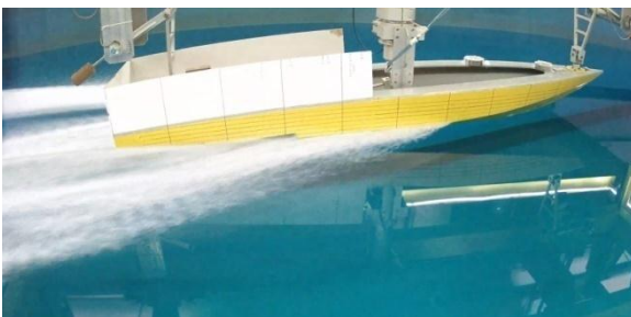
Figure 3. Cougar Model in NIMALA towing tank
