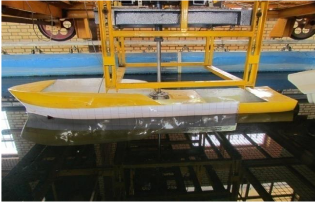
Figure 3. Ship model attached to dynamometer
