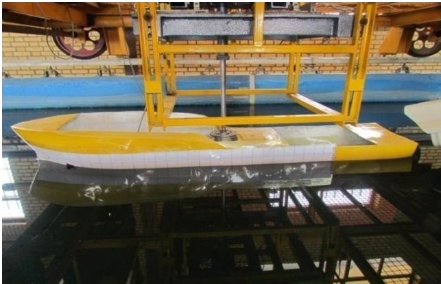
Figure 3. Ship model attached to dynamometer
