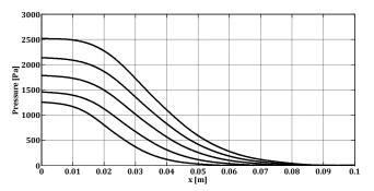
Figure 10. Air pressure over free surface for an ellipse and a wedge with  $\zeta = 3$  and  $V_0 = 1$  m/s at different time steps with  $\Delta t$ =0.15 ms.
