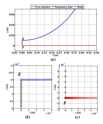
Figure 5. Mesh density on different boundary for an ellipse for with  $\zeta=3$  and  $V_0=1$  m/s, (a) half domain of the problem, (b) magnification of the mesh density at the intersection point of the body and the symmetry line, (c) magnification of the mesh density at the intersection point of the symmetry line and the free surface.
