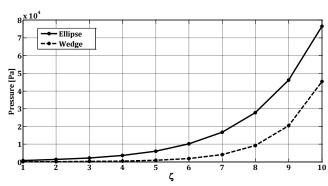
Figure 13. Variation of maximum cushioning pressure versus different  $\zeta$  with the same values of b.
