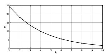
Figure 14. Variation of non-dimensional pressure ratio versus bluntness of the bodies
