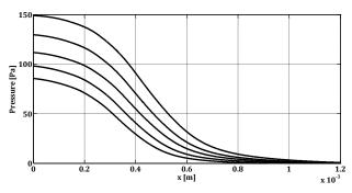
Figure 11. Air pressure over free surface for a wedge with  $\zeta = 3$  and  $V_0 = 1$  m/s at different time steps with  $\Delta t = 0.4$  ms.
