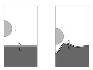
Figure 4. Schematic view of artificially divided surfaces in two different time steps
