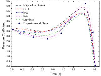
Figure 4. Comparison of the computed pressure coefficient with the experimental data Zhao et al. (1996) for different viscous models
