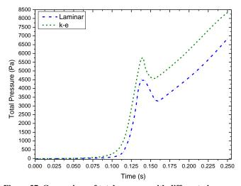
Figure 37. Comparison of total pressure with different viscous models
