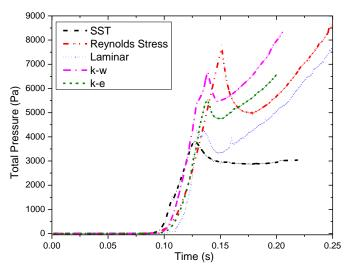
Figure 16. Comparison of total pressure with different viscous models
