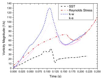
Figure 20. Comparison of vorticity with different viscous models
