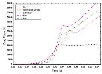
Figure 21. Comparison of drag force with different viscous models
