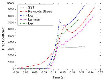
Figure 15. Comparison of drag coefficient with different viscous models
