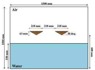
Figure 8. Geometrical configuration of the present study
