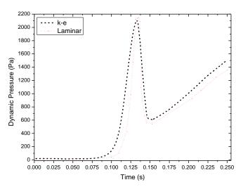
Figure 38. Comparison of dynamic pressure with different viscous models
