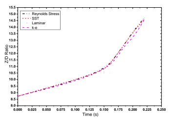
Figure 43. Comparison of Z/D ratio with different viscous models
