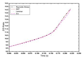
Figure 33. Comparison of  $\mathbf{Z}/\mathbf{D}$  ratio with different viscous models
