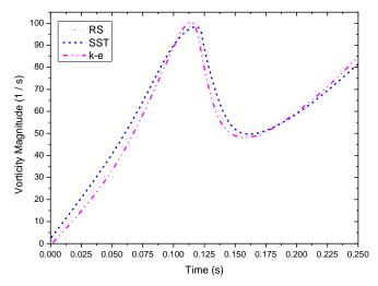
Figure 31. Comparison of vorticity with different viscous models
