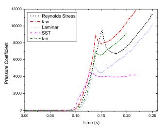
Figure 14. Comparison of pressure coefficient with different viscous models
