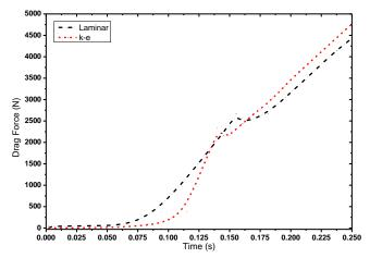
Figure 42. Comparison of drag force with different viscous models
