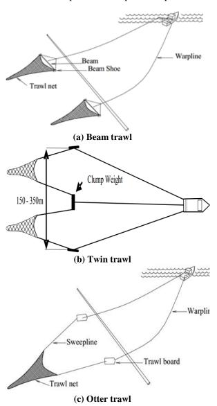
Figure 1. Different types of trawl gear [5].
