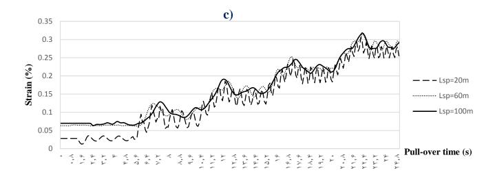
Figure 11. Submarine pipeline response under trawl gear pull-over load for Hsp=1 m: a) Displacement, b) Bending moment, and c) Strain.
