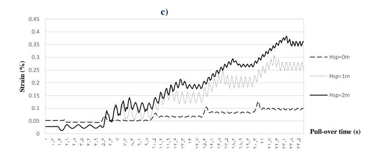
Figure 10. Submarine pipeline response under trawl gear pull-over load for Lsp=20m: a) Displacement, b) Bending moment, and c) Strain.
