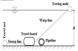
Figure 4. Trawl gear configuration, vertical plane.
