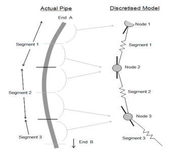
Figure 6. OrcaFlex line element model [19].
