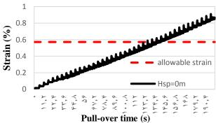
Figure 13. Comparison between Submarine pipeline response and design acceptance criteria trawl gear pull-over load for Lsp=100m.
