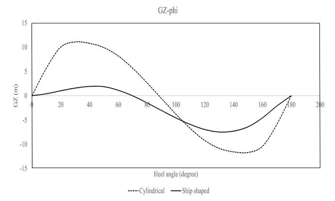
Figure (a). GZ- $\varphi$  diagram
