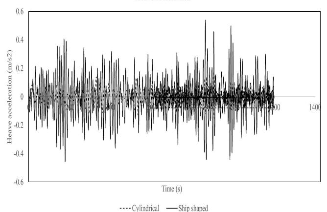
Figure (b). Heave acceleration comparison
