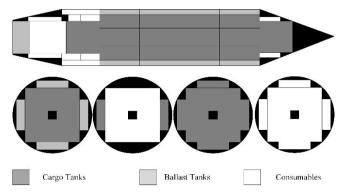
Figure 4. FPSO tank arrangement
