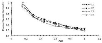
Figure. 11 Viscous to Pressure force ratio vs. Fr number for various side hull longitudinal position at Y1= 9.6 m.
