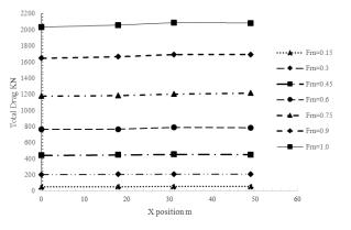
Figure. 9 The variation of total drag vs. x position of the side hull at Fr number when the transversal distance is Y1=9.6 m
