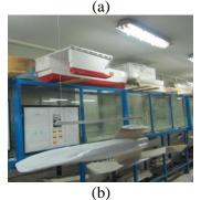
Figure. 2 (a) Application of the suspension method to determine the model's centre of gravity, (b) Application of Biffilar method for determination of radii of gyration
