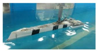
Figure. 6 Model during resistance test under head sea condition (model speed=0.5 m/s)
