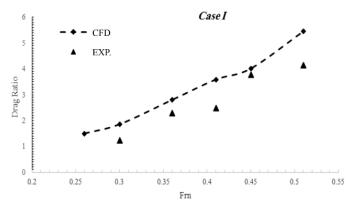
Figure. 7 The Drag ratio of case I for the data derived from the numerical approach and resulted from the experimental
