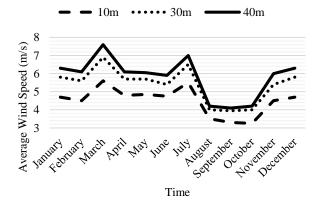
Figure 4 Monthly average wind speed at Bardekhun station [13]
