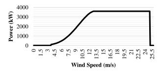
Figure 6 SWT 3.6 MW power curve [14]
