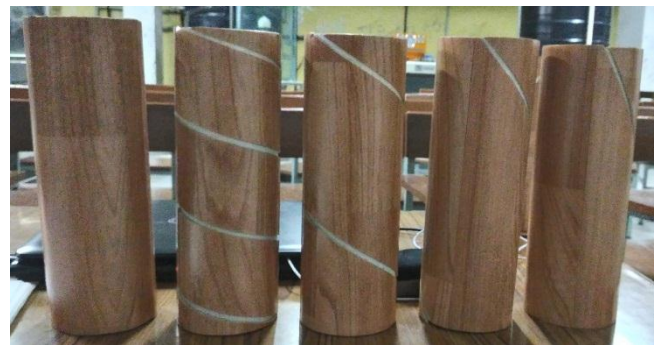
Figure 4. Smooth cylinder and groove cylinder of helix angle 15°, 30°, 45° and 60° respectively from left.
