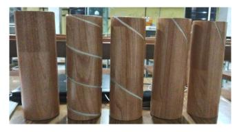
Figure 4. Smooth cylinder and groove cylinder of helix angle 15°, 30°, 45° and 60° respectively from left.
