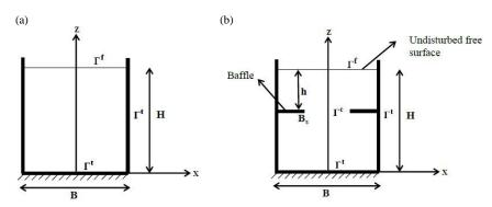
Fig. 1. Cross-section of rectangular container. a) Without baffle, b) with baffle.
