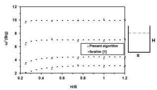
Fig. 2. Dimensionless sloshing frequencies for various liquid depths.
