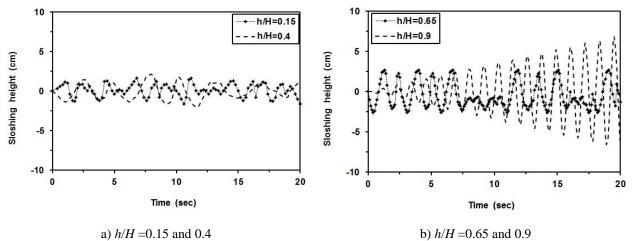
Fig. 7. Liquid sloshing height time histories for  $x_0$ =0.003m and various baffle positions.
