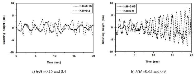
Fig. 8. Liquid sloshing height time histories for  $x_0$ =0.03m and various baffle positions.
