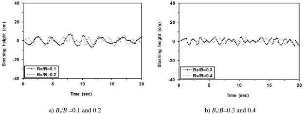
Fig. 9. Liquid sloshing time variations for various baffle widths.
