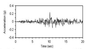
Fig. 12. Ground acceleration time history (1995 Kobe earthquake).
