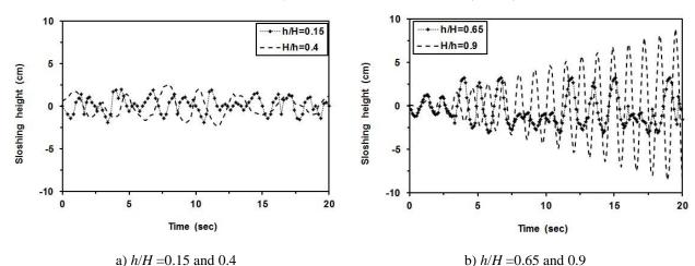
Fig. 10. Liquid sloshing height time variations for  $x_0$ =0.003m and various baffle positions.
