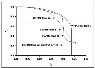
Figure 1. BS7910 failure assessment diagram
