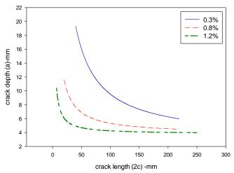
Figure8. Critical crack size curve according to FE based method for three strain levels (0.3%, 0.8%, 1.2%) for 16"pipe and 24mm wall thickness
