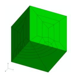
Figure 4. Standard quarter circular crack block [17]
