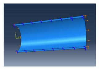
Figure 3. Fixed displacement at the un-cracked end of the pipe
