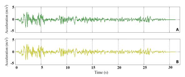
Fig. 10. Acceleration Time history of the Jacket Response under El Centro Excitation: (A) Before and (B) After Considering Added Deck Weight
