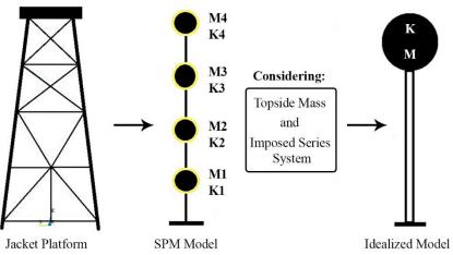
Fig.1. The SPM and the Idealized Model of the Jacket Platform
