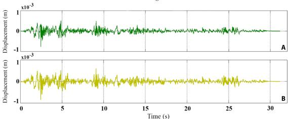
Fig. 11. Displacement Time history of the Jacket Response under El Centro Excitation: (A) Before and (B) After Considering Added Deck Weight
