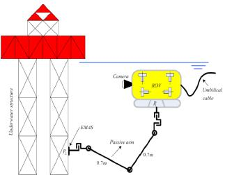
Figure 1. Dynamic positioning of an ROV with passive arm measurements [26]
