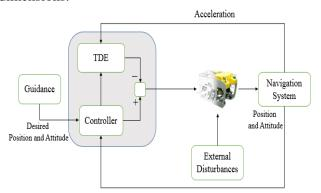
Figure 3. Block-diagram of control system
