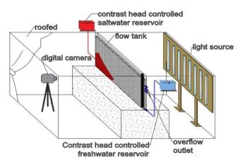
Figure 1. Schematic of the experimental set up.
