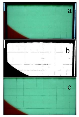
Figure 3. Pre-processing to remove areas outside the central chamber of the image. (a) Color image captured by camera, (b) Binary image, (c) Cropped image after masking.
