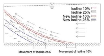
Figure 14. Schematic of expanding MZ. Due to flushing process, Dense Contour moves toward the sea boundary faster than dilute contour
