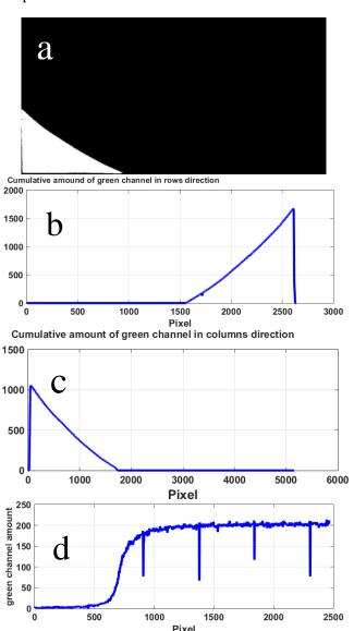
Figure 4. Data acquisition process. (a) Boundaries of SW in the HSI color space, (b) Horizontal projection of SW to determine  $h_{sw}$ , (c) Vertical projection of SW to determine  $L_T$ , (d) Variation of the green channel profile of the image to assess TMZ.
