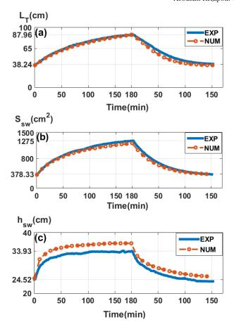
Figure 6. Transient behavior of SW (a)  $L_T$ , (b)  $S_{sw}$ , and (c)  $h_{sw}$  in the physical and numerical experiments. Advancing during 0< t< 180 min and receding t> 180 min
