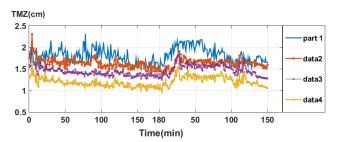
Figure 11. TMZ along the interface under transient condition in physical model
