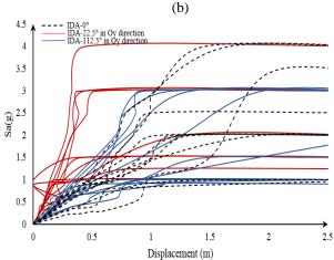
Figure 5. multi-recorded IDA (a) in 0, 22.5, and 112.5 degrees along Ox direction (b) in 0, 22.5, and 112.5 degrees along Oy direction.
