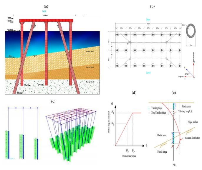
Figure 2. Maah-shahr wharf: (a) section (b) plan (c) Maah-shahr port in SAP2000 software. (d) moment-curvature curve of piles (e) distribution of plastic hinges on piles [19].
