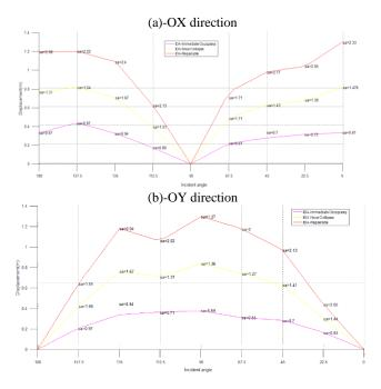
Figure 8. Summarized capacities of IDA in Ox and Oy directions for each incident angle.
