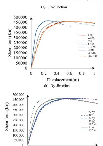
Figure 3. Pushover results of wharf No.1 in Maah-shahr port in (a) Ox-direction (b) Oy-direction.
