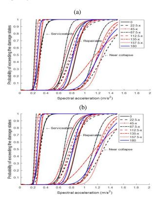
Figure 9. fragility curves in each incident angle for all damage sates (a) Ox direction (b) Oy direction.
