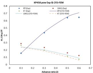
Figure. 13. Comparison of the hydrodynamic performances of KP458 POW composite propeller (CFD-FED) and rigid propeller (HMRI [23]).
