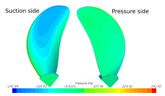
Figure. 15. Pressure distribution on flexible KP458 propeller surface at J=0.5 FSI simulation;
