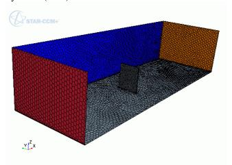
Figure. 3. Computational domain discretization by polyhedral mesh;
