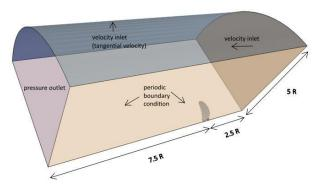
Figure. 8. Geometry of computational domain of KP458;
