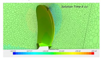
Figure. 11. Propeller shape deformation at J=0.6
