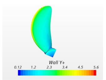
Figure. 10. Wall  $y^+$  distribution on the propeller blade at J=0.5;
