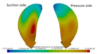
Figure. 14. Deformation distribution at J=0.5;
