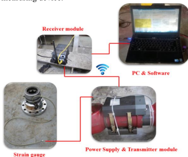
Figure 6. Schematic of torque measuring device
