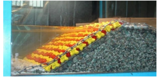
Figure 1 Geometry of breakwater built in the lab [16]
