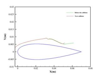
Figure 9 Track of bubble before and after impact with a wall with an initial radius of 50 μm.
