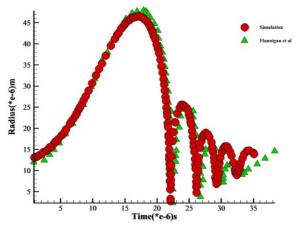
Figure 4 Comparison of Argon Bubble Behavior in Sulfuric Acid with Experimental Results of Flannigan et al.
