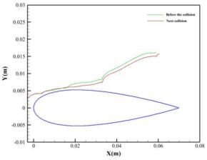
Figure 15 Track of a bubble with an initial radius of  $100~\mu m$  before and after colliding with another bubble with an initial radius of  $100~\mu m$
