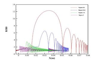
Figure 7 Graph of radius changes after colliding with a wall along the bubble travel path for different cavitation numbers for an initial radius of 100 µm
