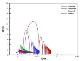
Figure 6 Graph of radius changes along the bubble motion track for different cavitation numbers for an initial radius of  $100~\mu m$
