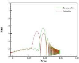
Figure 10 Bubble radius before and after impact with the wall with an initial radius of 100  $\mu m$ .
