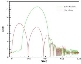
Figure 12 Bubble radius before and after impact with the wall with an initial radius of 200  $\mu m$ .
