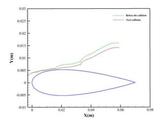
Figure 16 Track of a bubble with an initial radius of 100 µm before and after colliding with another bubble with an initial radius of 200 µm
