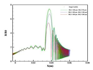
Figure 14 Comparison of bubble radius in the collision of two bubbles in a single state and the presence of bubble with initial radii of  $50 \mu m$ ,  $100 \mu m$ , and  $200 \mu m$ .
