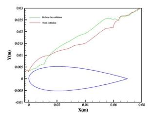
Figure 13 Track of bubble before and after impact with a wall with an initial radius of 200  $\mu$ m.
