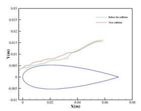
Figure 11 Track of bubble before and after impact with a wall with an initial radius of 100  $\mu$ m.
