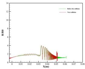
Figure 8 Bubble radius before and after impact with a wall with an initial radius of 50 µm.
