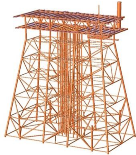
Figure 5. Jacket Modeling in SACS Software
