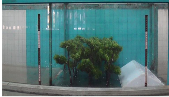
Figure 1- Tree-structure arrangement in the laboratory flume
