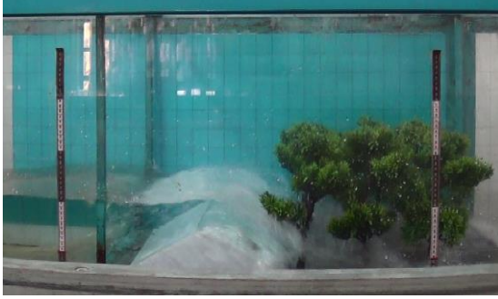
Figure 1- Tree-structure arrangement in the laboratory flume
