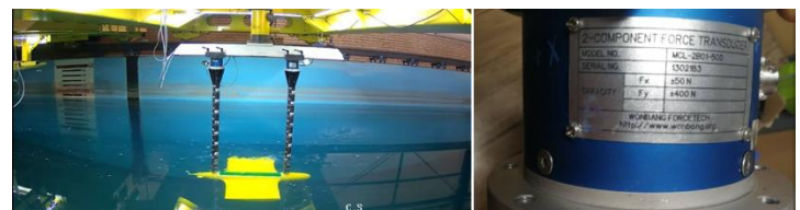
Figure (3): A view of the NIMALA towing tank and model test attachment to the struts and 2-component force transducer
