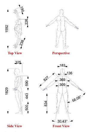
Figure 3. Main Geometry Dimension and Specifications
