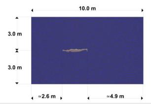
Figure 7. Figure 6. Domain and Boundary Condition Side View
