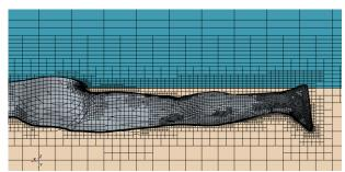
Figure 9. Trimmed Cell Mesh Implemented on Geometry No.1.
