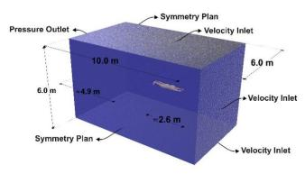
Figure 5. Domain and Boundary Condition Prespective View
