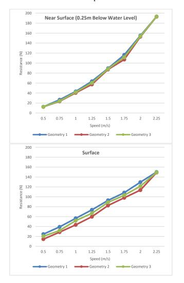
Figure 17. Resistance vs Speed Diagram for Different Swimming Positions.
