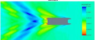
Figure 9. Wave contour at 20 knots speed
