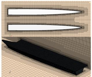
Figure 5. Computational mesh on the ship
