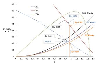
Figure 14. Kt, Kq, Eta, J diagram of propeller
