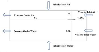
Figure 4. Computational Domain and Boundary Condition
