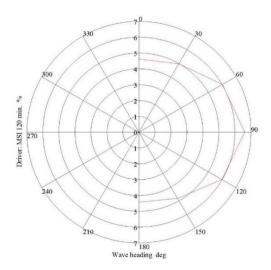
Figure 39: Polar Diagram of MSI Seasickness for a 2-hour Duration for the Driver's Seat at a Trim Angle of 0
