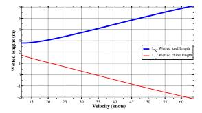
Figure 43: Length of keel line and wetted beam at the initial trim angle of 6.0 degrees and LCG=1.483 m.
