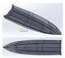
Figure 4: Accurate 3D scanning of the boat in water (final model).
