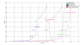
Figure 14: Curves of Variation in Hull Form
