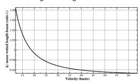
Figure 44: Ratio of average wetted length to beam width at the initial trim angle of 6.0 degrees and LCG=1.483
