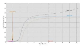
Figure 26: Float RAO for a static trim angle of 0 degrees at a wave incident angle of 180 degrees.
