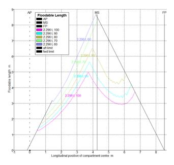
Figure 17: Length of Flooding vs. Different Penetration Coefficients
