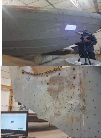
Figure 1: Marking points on the boat hull and scanning different sections of the boat on dry land.
