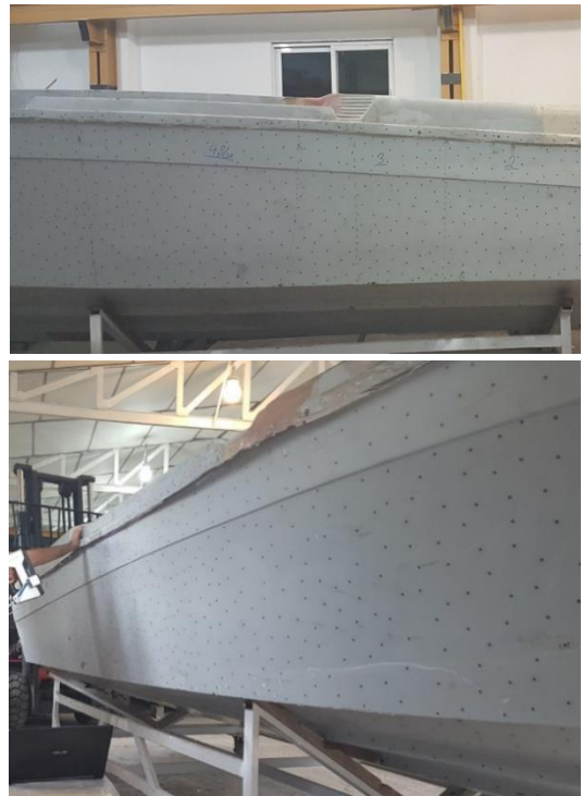
Figure 3. Scanning of the left and right sides of the boat
