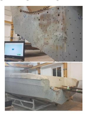
Figure 4. Scanning of the hull bottom and transom
