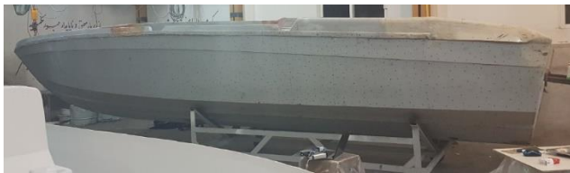
Figure 1. Marking points on the entire hull of the boat on the first day
