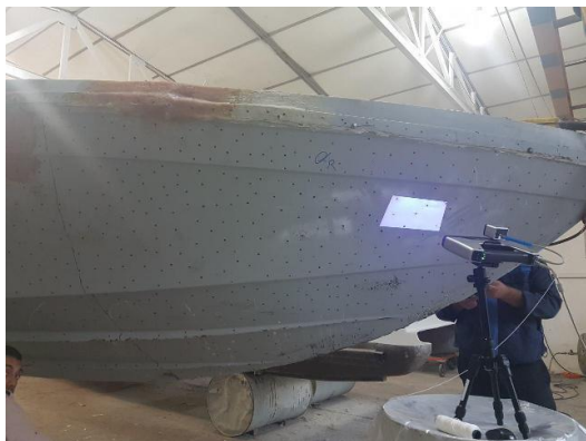
Figure 2. Scanning of the front section of the boat
