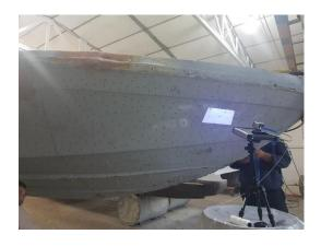
Figure 2. Scanning of the front section of the boat
