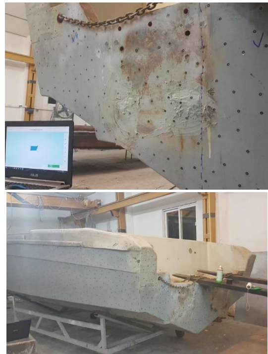
Figure 4. Scanning of the hull bottom and transom
