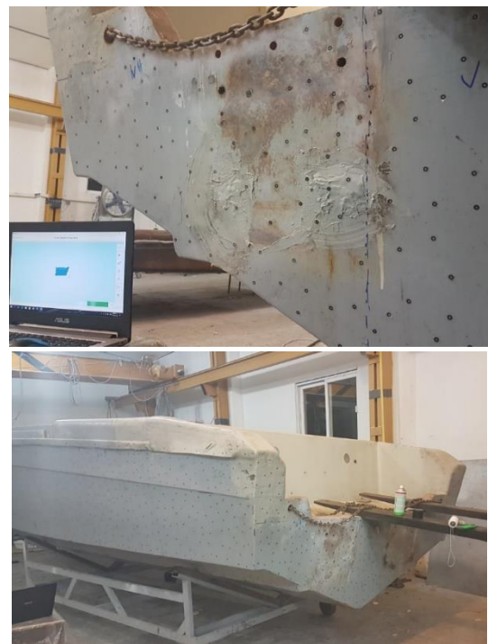
Figure 4. Scanning of the hull bottom and transom
