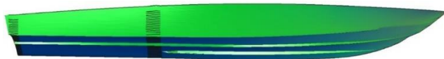
Figure 20. Side view of the hull modeling using triangular mesh in the Maxsurf environment.
