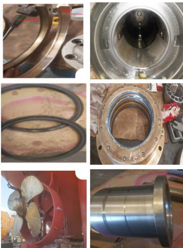
Figure 12. Stern tube aft ring seal box [13].
