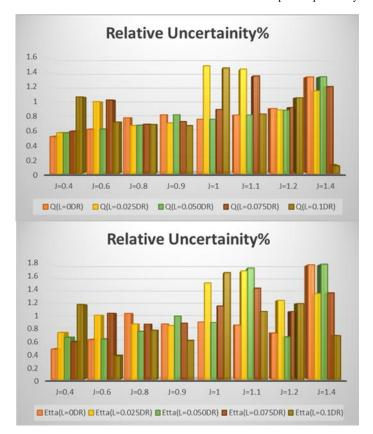
Figure 13: Comparative Bar Chart of the Percentage Relative Uncertainty for Duct and Stator Assembly Thrust, Rotor Thrust, Total Thrust, Rotor Torque, and Open waterEfficiency for Five Investigated Conditions at Various Advance ratios.
