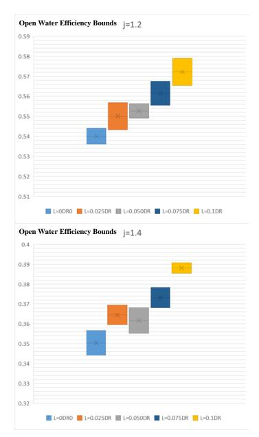
Figure 17: Comparative Bar Chart of Openwater Efficiency Ranges for Five Investigated Cases at Various Advance Ratios
