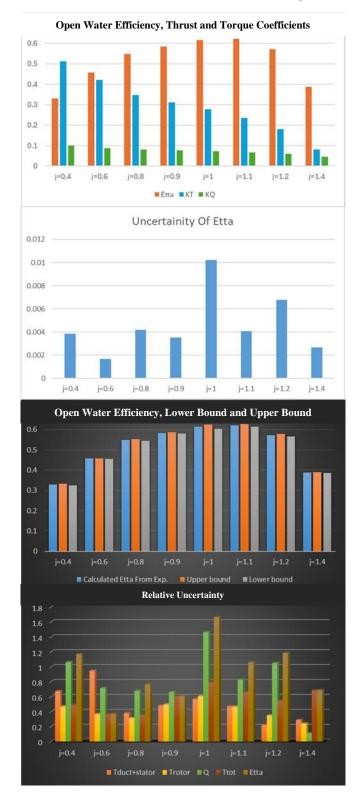
Figure 12: Bar chart arrangement. Up to down: Efficiency plot, thrust and torque coefficients, open water efficiency uncertainty plot, Open water efficiency values with upper and lower bounds; relative uncertainty plot for duct and stator thrust, rotor thrust, total thrust, rotor torque, and open-water efficiency parameters (in percentage terms) across different advance ratios for the L=0.01DR configuration.
