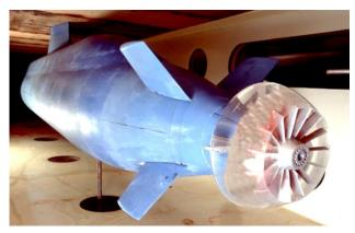
Figure 1. Pump jet on submarine model in the cavitation tunnel at SSPA [2]
