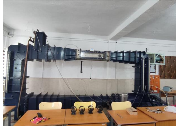
Figure 4: View of the Cavitation Tunnel at Imam Khomeini Naval University (Noshahr)
