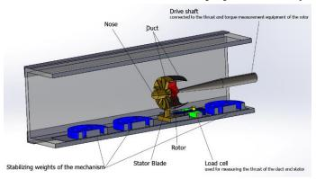
Figure 6: Installation Method of the Propeller Assembly in the Cavitation Tunnel
