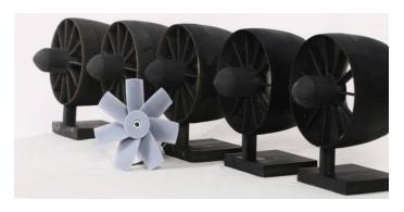
Figure 5: Five Geometries Fabricated for Experimental Testing
