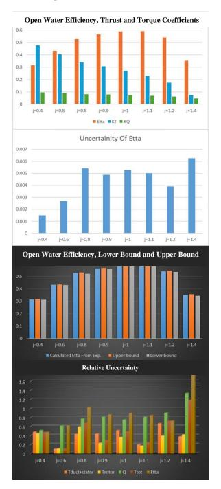
Figure 8: Bar chart arrangement. Up to down: Efficiency plot, thrust and torque coefficients, open water efficiency uncertainty plot, Open water efficiency values with upper and lower bounds; relative uncertainty plot for duct and stator thrust, rotor thrust, total thrust, rotor torque, and open-water efficiency parameters (in percentage terms) across different advance ratios for the L=0DR configuration.
