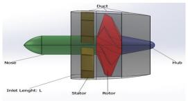
Figure 3: Component Diagram of the Pre-swirl Jet Pump
