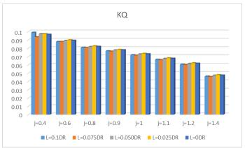
Figure 15: Comparative Bar Chart of Torque Coefficient for Five Investigated Conditions at Various Advance ratios.
