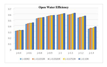
Figure 16: Comparative Bar Chart of Open water Efficiency for the Five Investigated Cases at Various Advance ratios.
